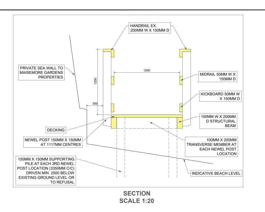
NEWEL POST 150MM X 150MM AT 1117MM CENTRES 100MM X 200MM 150MM X 150MM TRANSVERSE SUPPORTING PILE AT MEMBER AT EACH 3RD NEWEL POST **EACH NEWEL** LOCATION (3350MM C/C) POST LOCATION 1117MM C/C DECKING 100MM W X 200MM D STRUCTURAL BEAM
